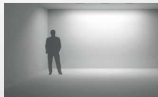
Wall washing Lighting
